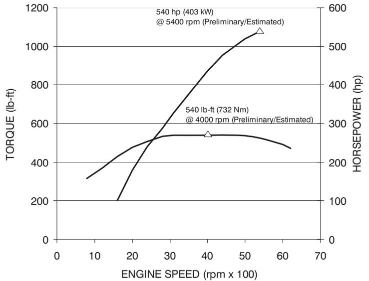
Actual power levels may vary depending on OEM calibration and application. Plot depicted represents Marine "LSA" engine as tested with Premium Fuel (Preliminary/Estimated values).
